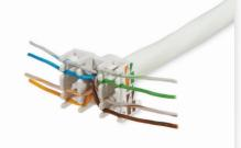
Lay the wires to their correct positions based on the color code (T568A/T568B)
